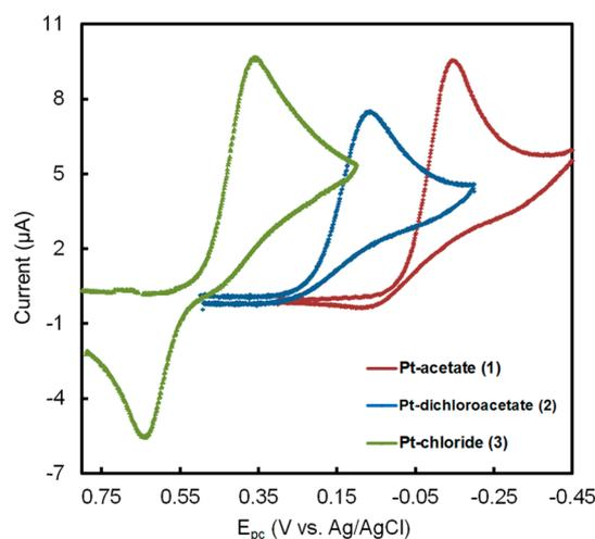
**Figure 1.** Background subtracted cyclic voltammograms of prodrugs **1–3** at  $0.1$  V s<sup>-1</sup>.
