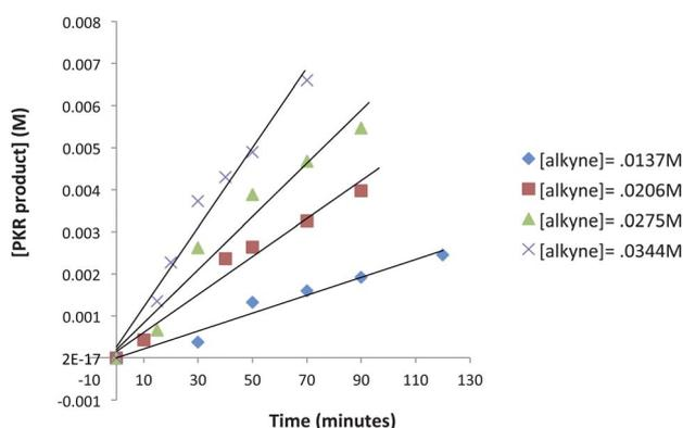
Fig. 6 Reaction profile dependence on alkyne concentration in regions which display linear behavior (an average of three experimental iterations).
