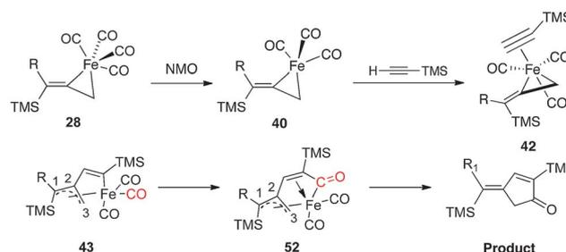
**Fig. 17** Mechanistic pathway of the iron-mediated PKR.
