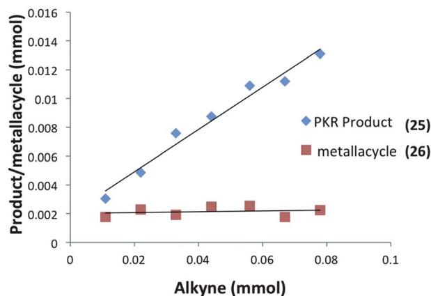
**Fig. 5** Conversion of allene into PKR product **25** and metallacycle **26** as a function of alkyne concentration (an average of three experimental iterations).
