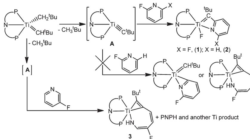
**Scheme 3** Synthesis of complex **1** and **2** by C–F activation, as well as the fluorosubstituted ring-opened product, **3**.
