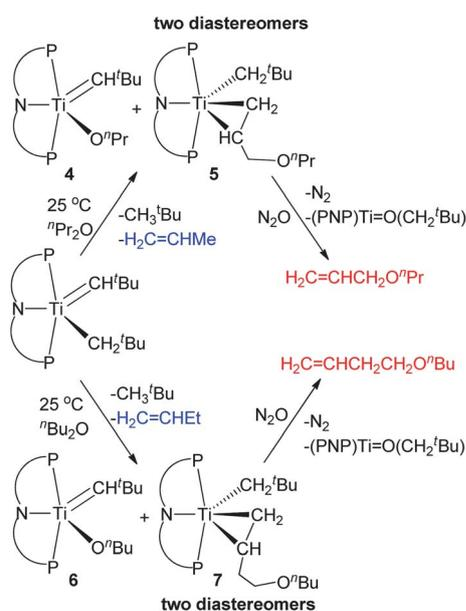
**Scheme 4** Dehydroalkoxylation and dehydrogenation of  $^n\text{Pr}_2\text{O}$  and  $^n\text{Bu}_2\text{O}$  by complex  $(\text{PNP})\text{Ti}=\text{CH}^t\text{Bu}(\text{CH}_2^t\text{Bu})$ .
