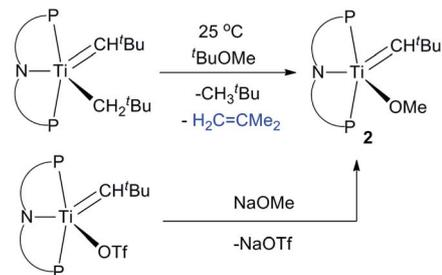
**Scheme 2** Dehydroalkoxylation and dehydrogenation reactions involving (PNP)Ti=CH<sup>t</sup>Bu(CH<sub>2</sub><sup>t</sup>Bu) and <sup>t</sup>BuOMe.
