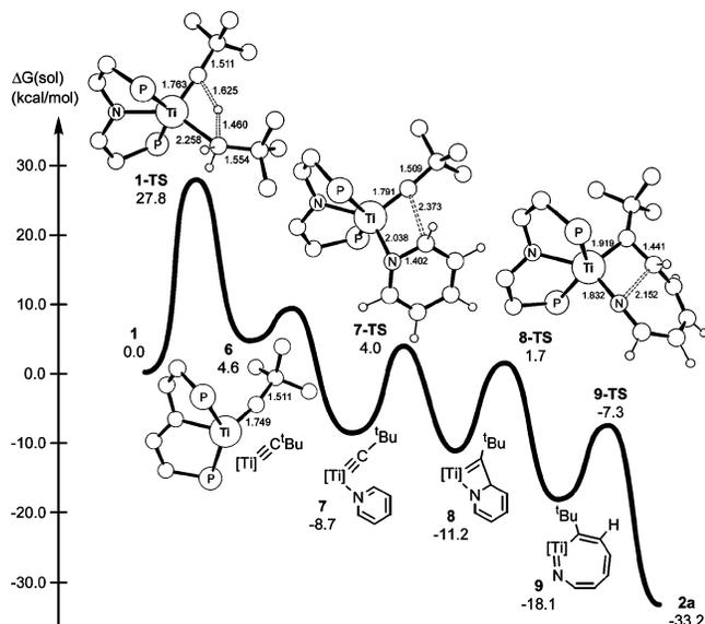
**Figure 2.** Proposed mechanism of the ROM of pyridine. Only core structures are shown for illustration. All energies are solution phase free energies, and all bond lengths are given in Å. [Ti] represents the (PNP)Ti framework, and solvation calculations were carried out at the optimized gas-phase geometry employing the dielectric constant of  $\epsilon = 2.379$  (pyridine).
