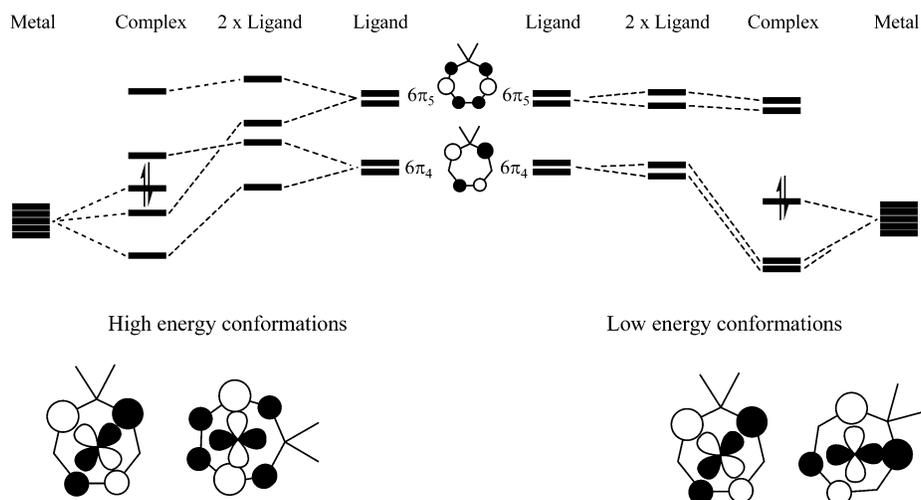
**Figure 6.** Schematic diagram of the frontier orbitals in Mo66, shown in the high-energy ring conformations (points A and C) and low-energy conformations (points B and D). The HOMO is indicated with two electrons. Shown in the center are the empty ring orbitals of  $\delta$ -symmetry, which combine and interact with the metal  $d_{xy}$  and  $d_{x^2-y^2}$  orbitals. In high-energy conformations the unfavorable  $6\pi_5$  orbital must be used.
