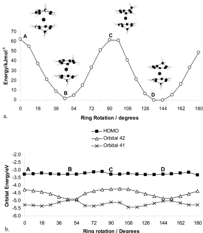
**Figure 5.** Energy profile for ring rotations of Mo66 through 180°: (a) total energy; (b) energy of occupied orbitals HOMO, orbital 42 (HOMO-1), and orbital 41 (HOMO-2).
