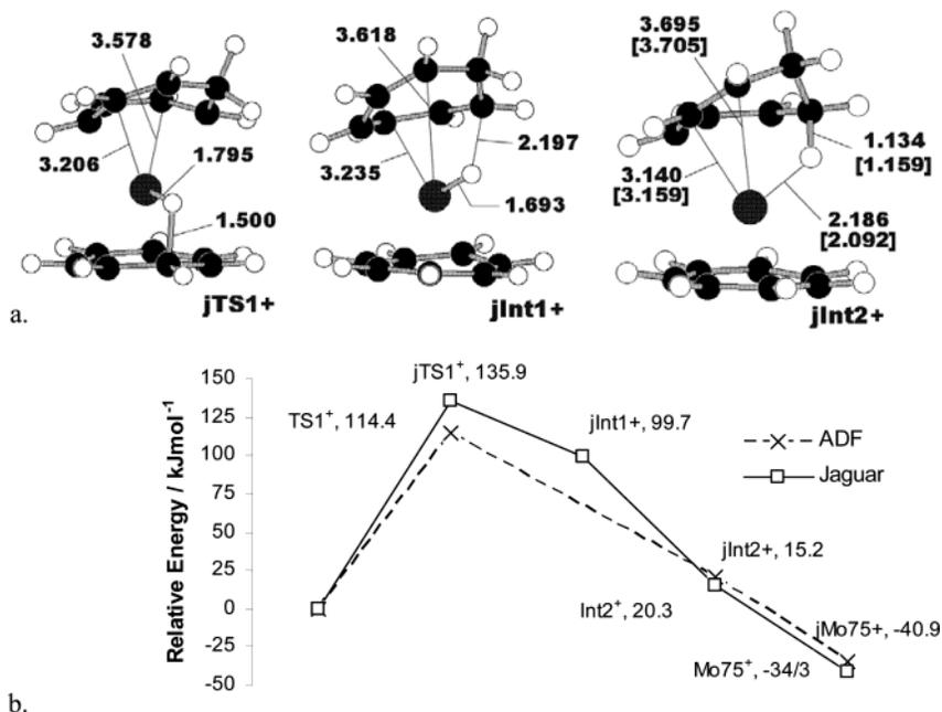
**Figure 9.** (a) Stationary points found in the conversion of  $j\text{Mo}66^+$  into  $j\text{Mo}75^+$ . Distances for ADF stationary points are labeled in square brackets. Distances shown are for the metal to migrating hydrogen, and metal to decoordinated carbon atoms. (b) Relative free energies for the structures shown in (a).
