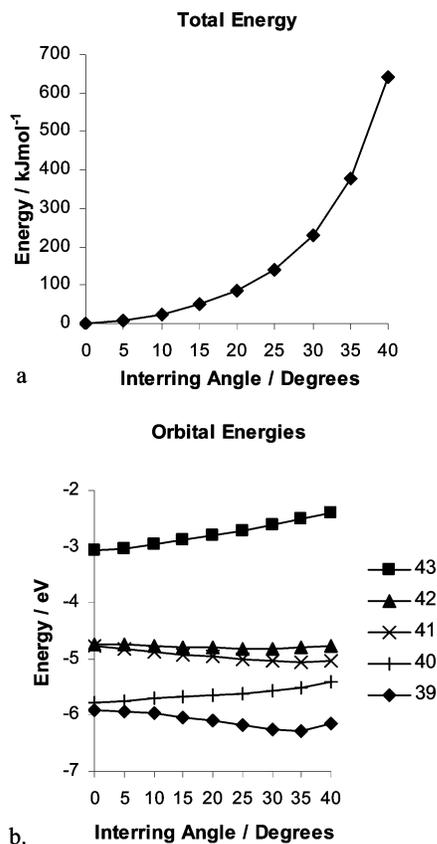
**Figure 4.** Effect of varying  $\gamma$  ( $180^\circ$  – angle between metal atom and two ring centroids) in Mo66 on (a) the total energy and (b) orbital energies.
