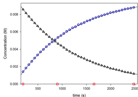
**Figure 3.** Amidation profile at  $-47.7\text{ }^{\circ}\text{C}$ : black triangle, [**1-Ir**]; blue circle, [**4-Ir**]; red square, [**4-Rh**]. Data were fit ( $R^2 = 0.999$ ) to first-order exponential decay.
