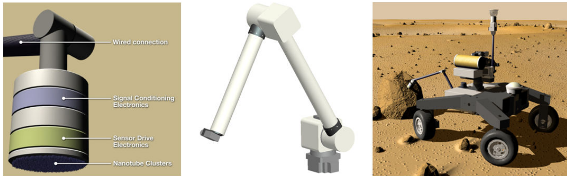
Fig. 65. Artistic rendering of biosensor and supporting equipment (left), engineering model of the arm in development (center), and artistic rendering of \Psi executing the demonstration with the biosensor (right).
