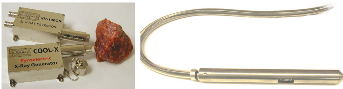
Fig. 66. COTS X-Ray source and detector (left), and the flight qualified borehole XRF probe (right).
