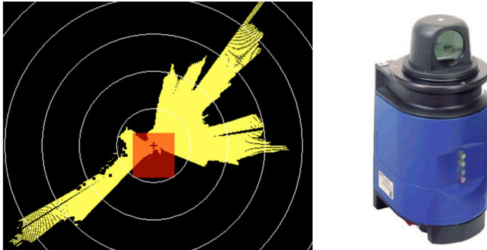
Fig. 13. Data taken by the laser-range finder as it is displayed to the user (left), and the SICK LD-OEM1000 scanning-laser range-finder (right).
