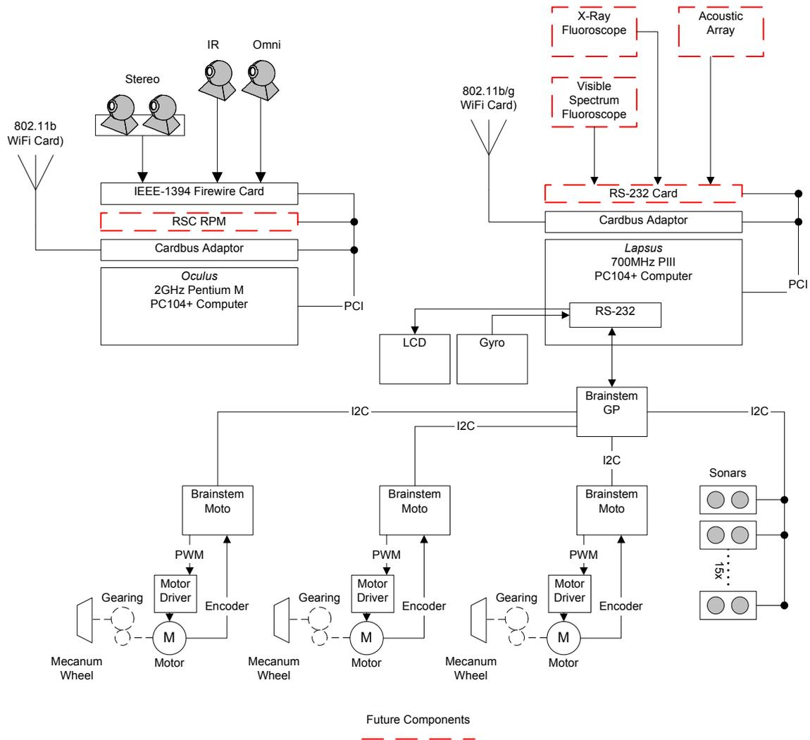
**Figure 5 Electrical-hardware architecture**
