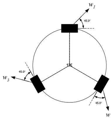
**Figure 3 Tangential velocity vector components.**
