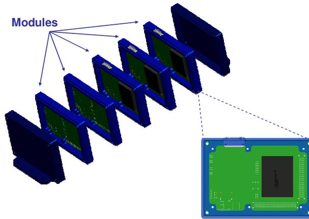
**Figure 8 Exploded view of RSC stack**
