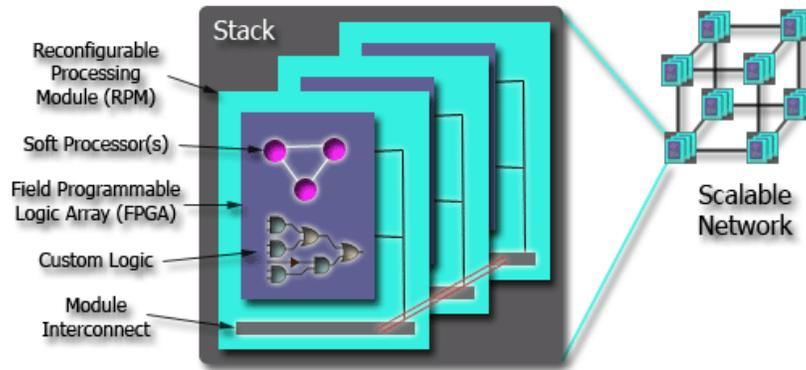
**Figure 7 High-level RSC architecture**
