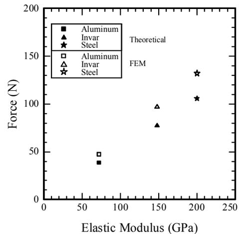
**Figure 6. FEM and theoretical transverse forces for the three alloys. A  $25\mu\text{m}$  range of motion is used for these simulations**
