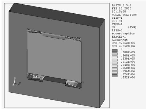
Figure 4. 3D eight-node structural solid element mesh of the four flexural hinges of the guided-motion nanopositioner stage of Figure 1. BC's are prescribed on the four corners.
