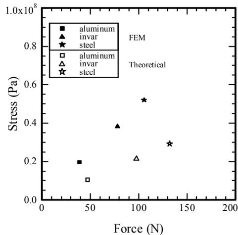
**Figure 7. Stresses versus transverse forces in the hinges. A 25  $\mu\text{m}$  range of motion is used for these simulations.**
