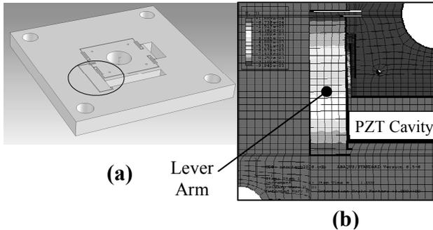
**Figure 5. The positioner structure with the lever arm a) as modeled in SolidWorks, and b) as analyzed in ABAQUS**
