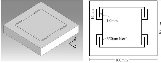
**Figure 1. A flexural-hinge guided-motion. The outer frame is secured to a footprint and a probe or a device is secured to the inner stage. The PZT actuator is housed in a cavity in the bottom of the stage. (not shown)**
