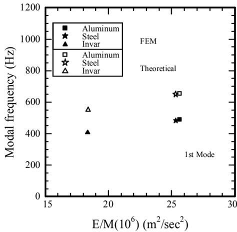
Figure 2. 1<sup>st</sup> modal frequency for the three alloys, aluminum, stainless steel, and invar.
