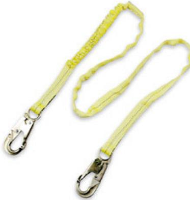
*The Shock Absorbing Lanyard employs a unique webbing technique which allows a controlled stretch during fall arrest, thus reducing the shock to the wearer, as much as 50% over corresponding 5/8" nylon rope lanyards. When the shock absorbing lanyard receives a force of 600 lbs. exerted on it, an indicator flap pops out to indicate the lanyard has been subjected to a fall, and the lanyard is **NOT TO BE REUSED!!!***
