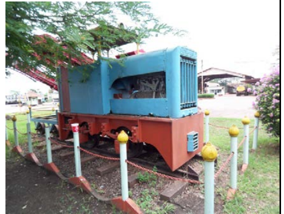
Hudson-Hunslet 0-4-0 N°2271 built 1940 with Gardner 4 cyl. diesel engine N°74186 750mm gauge
