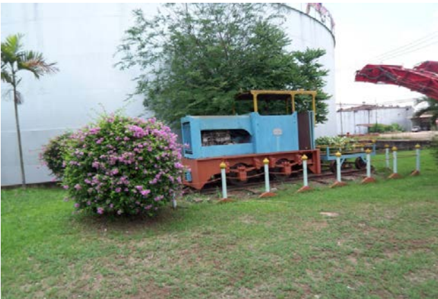
Hudson-Hunslet 0-4-0 N°2271 built 1940 with Gardner 4 cyl. diesel engine N°74186 750mm gauge
