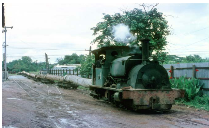
No.8 Hudswell Clarke 0-4-2ST No.900 built 1909 with a full load of logs mounted on pairs of 4-wheeled bogies, trundles its way to the sawmill in 1971.
