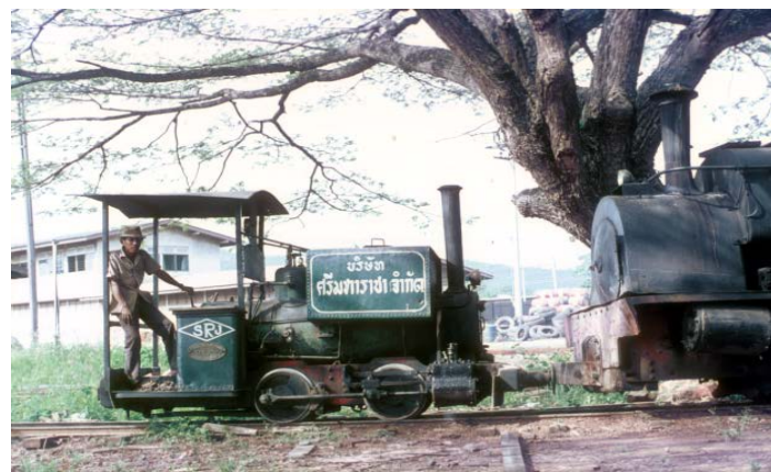
No.2 Kerr Stuart 0-4-0ST No.2387 built 1915 was the pride & joy of the mill and performed shunting duties in the yard, restricted in its range due to its small wheels. Ex-Borneo Co. Now preserved at the Siam Country Club
