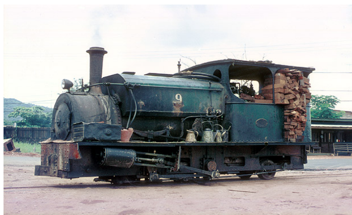
No.9 Hudswell Clarke 0-4-2ST No.367 built 1890 in steam at the sawmill in 1971. By far the oldest surviving locomotive in Thailand , at that time. Where is it now ? Ex-Borneo Co.
