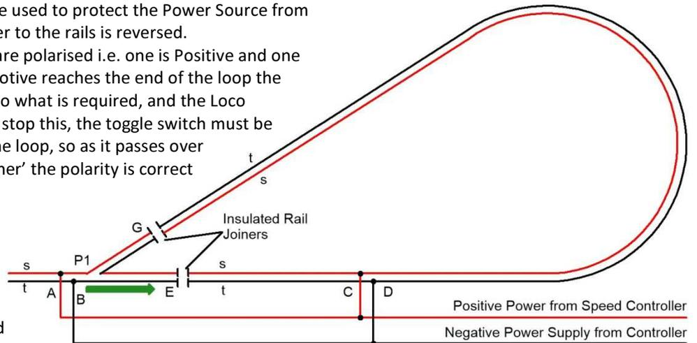
**Note:** The polarity of the loop never changes, it's the main line that is changing polarity. In the drawing below the Locomotive is now in the position of the Green Arrow. The DPDT switch must be thrown before it reaches the 'Insulated Rail Joiners' G. This will change the polarity of the main track after the 'Rail Joiners' G. As you have an Insulated track joiner at 'E' this change will have no effect on the Loop Polarity.
