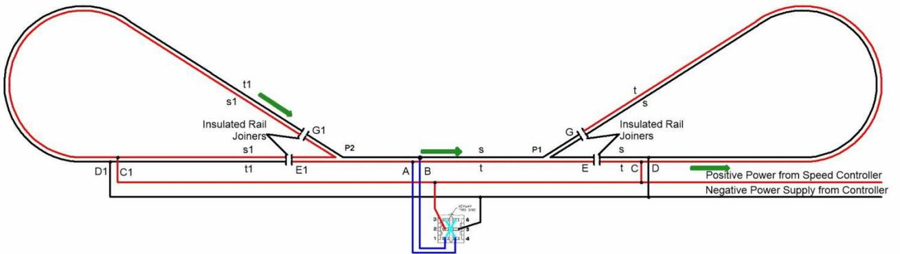
The next drawing shows the polarity has changed to allow the train to pass through points P1, run along the straight to points P2. The points P2 have also changed to allow the train to pass onto the lower part of the left loop. The process starts again
