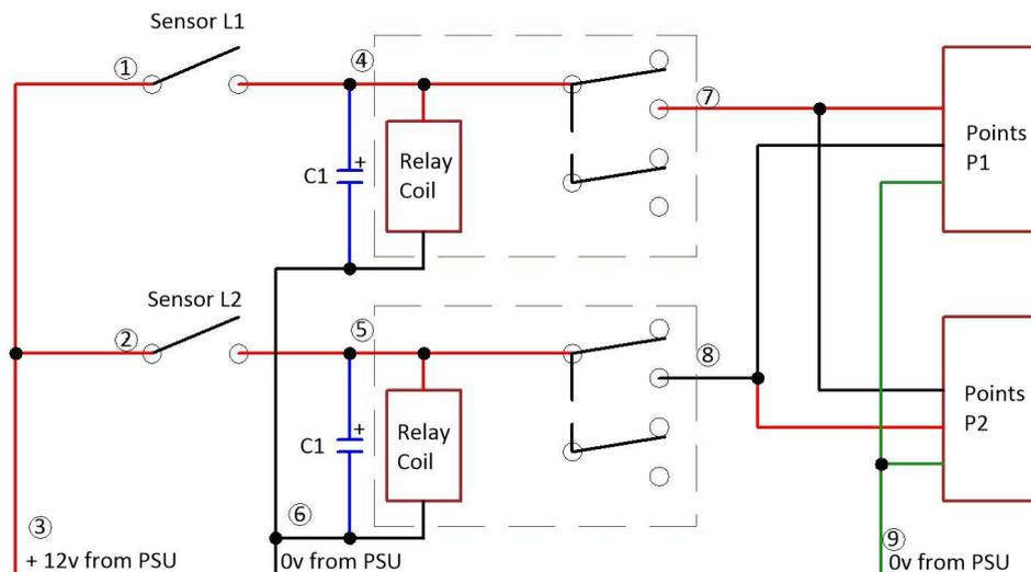
The drawing below shows the complete layout for the fully automatic Reverse Loop. The numbers in circles on the circuit above have been transposed to the layout below.
