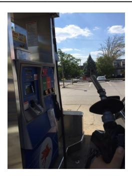
The design of the nozzle of the pump is an affordance that tells the user that the pump needs to be inserted into the gas tank of the car. The nozzle also is designed with a piece of rubber to prevent the user from inserting the nozzle too far into the gas tank. The long rubber hose that connects the pump is also an affordance that tells the user how close he or she should park next to the pump, and constrains the user from parking too far away.
