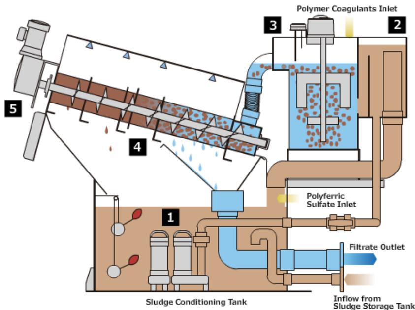
Sludge is pumped into a blending tank where coagulant is added. The mixture then flows to a flocculation tank where by means of polymer, the pollution is concentrated into flocs and as much as possible free water is created.
