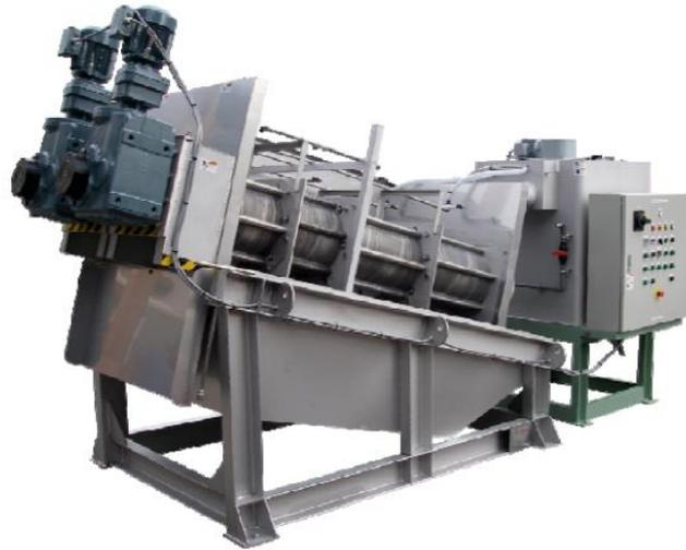
The dewatering drum is an assembly of fixed and moving rings. The movement of the screw causes the rings to move against each other and with this motion actively clean off the dirt in the apertures between the rings.
