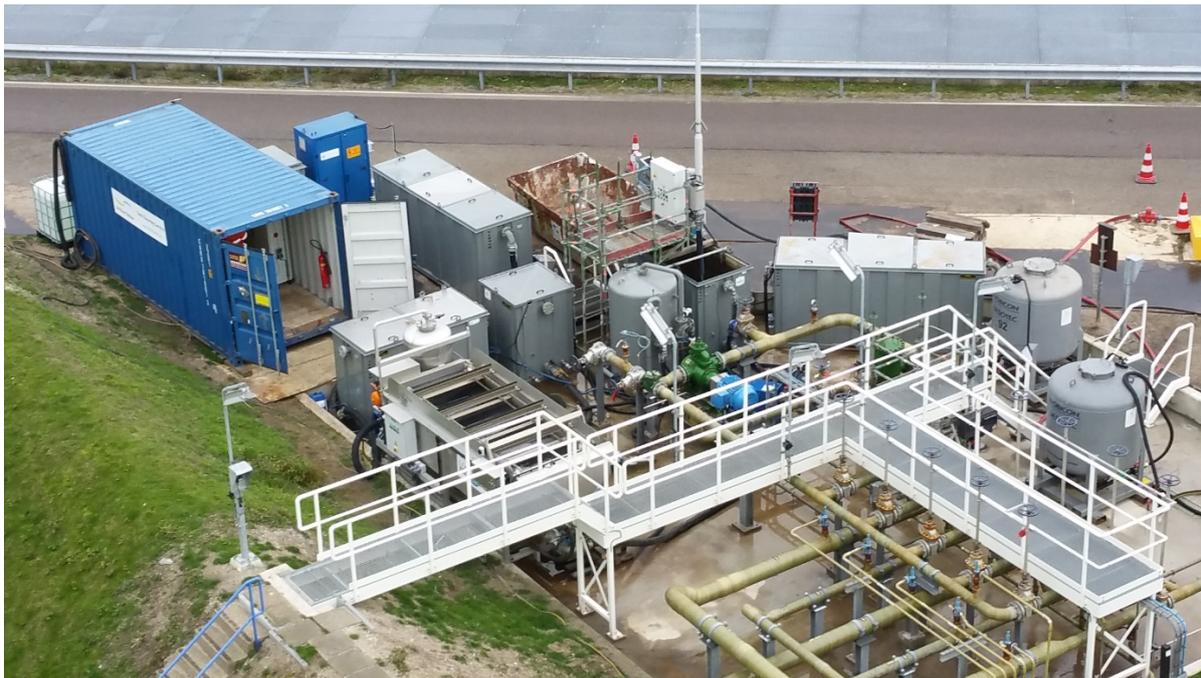
The MicroZapp media loading was 300-400 micron with a bed depth of approximately 70 cm. The flow rate was 8-10 m<sup>3</sup> per m<sup>2</sup> of filter area and the job lasted for 6 weeks.
