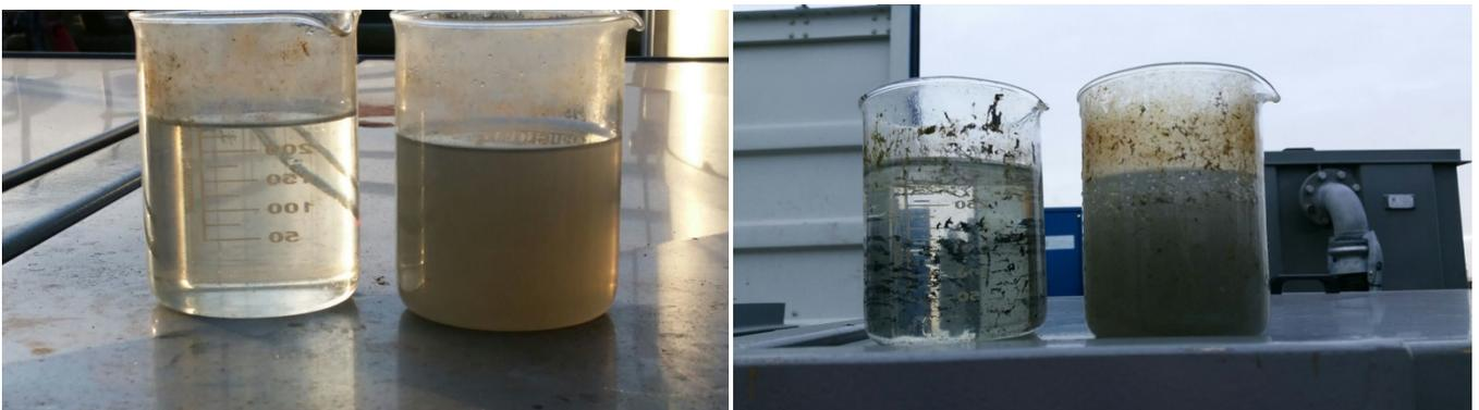
Normal filter feed and results with around 1.0 to 1.5 bar differential pressure
