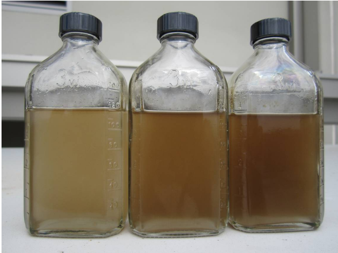
Figure 9: Samples: Underflow with DCC / underflow without DCC / Inlet of HC.
