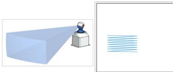
**Region Scanning** — This mode allows the user to define a rectangular region within the scanner's azimuth and elevation field in which to concentrate the scanning. The Region Scan mode gives the most control over the attention of the scanner with scan rate, number of lines per degree, sample rate and sample averaging parameters available as in other modes. Region Scanning is most useful when a region's extent in azimuth is less than 60°.
