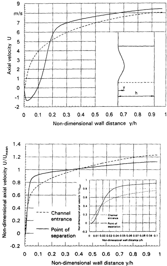
Figure 6. Velocity profiles just upstream and downstream of the wave for case 12-6.
