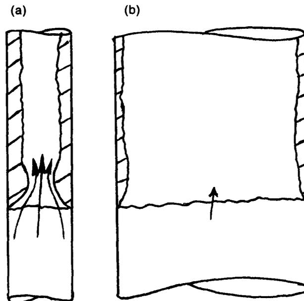
Figure 14. Shape of the hanging film reported by Wallis & Makkenchery (1974): (a) in small diameter tubes and (b) in large diameter tubes.
