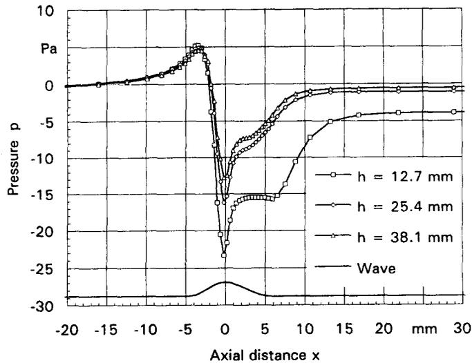
Figure 9. Effect of channel height on the wall pressure profile for a gas velocity of 6.3 m/s.
