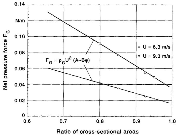
Figure 12. Correlation of the force on the wave as a function of the ratio of cross-sectional area.
