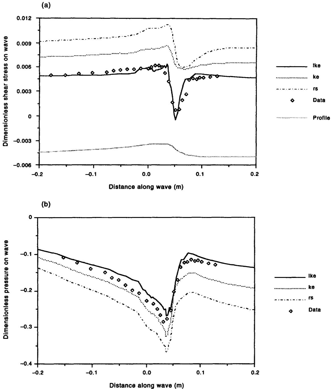
Figure 3. Variation of (a) non-dimensionalized static pressure and (b) non-dimensionalized shear stress induced by gas flowing over a roll wave. The squares are the data of Miya (1970) and the predictions of the standard  $k-\epsilon$  model (ke), the Reynolds stress model (rs) and the low Reynolds number  $k-\epsilon$  model (lke) are shown. The flow Reynolds number is 23,400.
