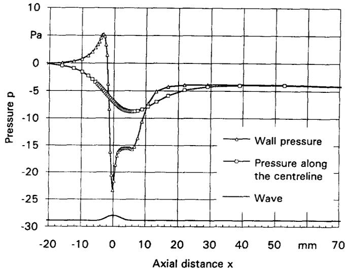
Figure 7. Variation of static pressure in the channel for the case of 12-6.
