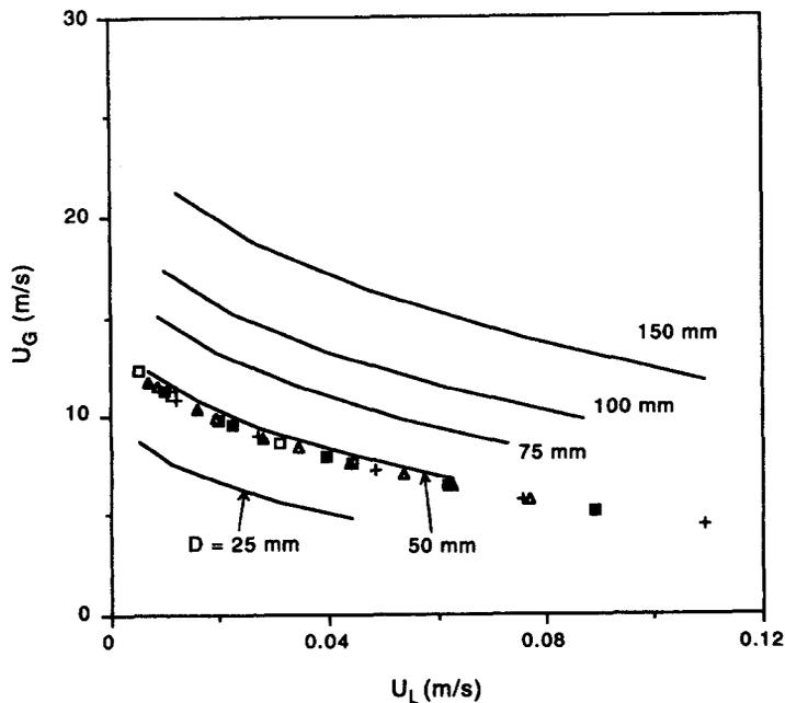
Figure 1. Comparison of the gas velocity required for flooding predicted by the Wallis type of correlation (lines) with that predicted by the Kutateladze type of correlation (squares etc.) for typical liquid velocities and for various tube diameters. The figure shows that the two correlations agree for a tube diameter of 50 mm.
