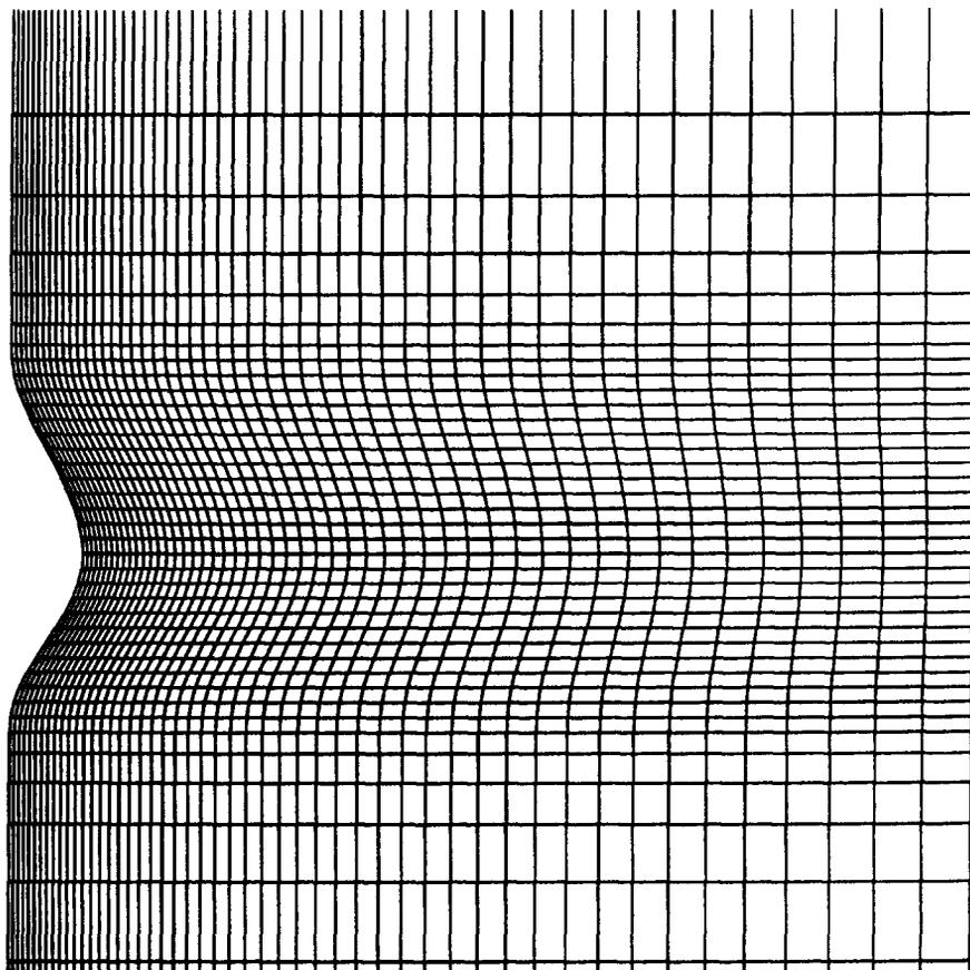
Figure 4. Typical grid used in the calculations with a uniform expansion factor in a  $y$ -direction of 1.05.
