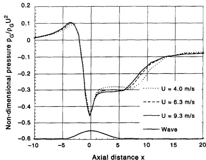
Figure 10. Effect of gas velocity on the pressure profile for a channel half-height of 12.7 mm.
