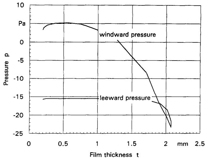
Figure 11. Pressure on the windward and the leeward sides of the wave for the case of 12-6.
