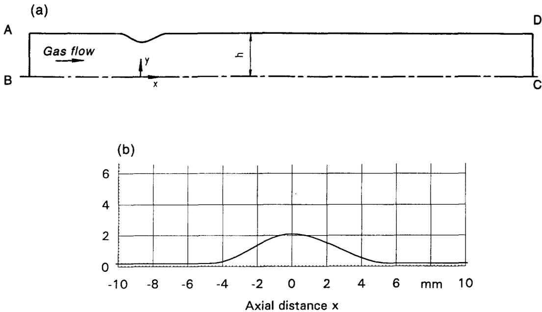
Figure 2. Formulation of the problem: (a) flow domain and boundary conditions and (b) detail of the standing wave.
