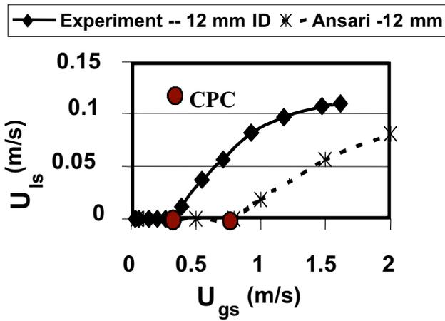
Figure 11 Comparison of laboratory data and model prediction of liquid production rate ( $D=12$  mm,  $h=63.5$  cm)
