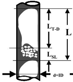
**Figure 1** Schematic of slug flow features frequently observed with conventional gas lifting
