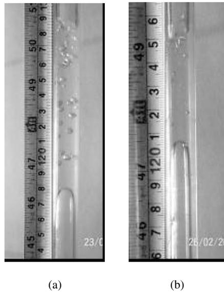
Figure-9 (a) pseudo slug flow pattern with water only (D=12 mm, h=63.5 cm  $U_{gs} = 0.54$  m/s  $Q_g = 3.7$  l/min) (b) train-of-bubbles with water-methanol (D=7.8 mm, h=63.5 cm,  $U_{gs} = 0.21$  m/s,  $Q_g = 0.6$  l/min,  $\sigma = 38$  dyne/cm)
