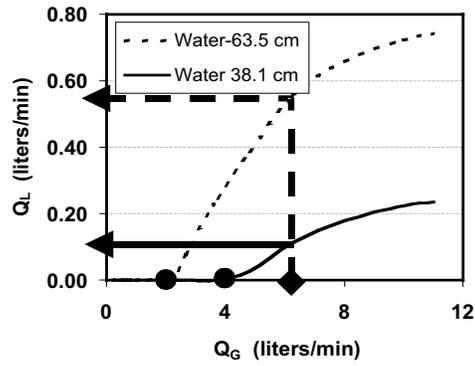
**Figure 4** Influence of reservoir pressure on the liquid production rate (production characteristics for  $D=12\text{mm}$  and  $h= 63.5$  and  $38$  cm - water only)
