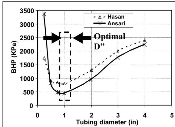
**Figure 2** The effect of tubing diameter on the bottom hole pressure required for sustaining a fixed liquid production rate (numerical models) [ $H=200\text{m}$ ,  $Q_L=1\text{BBD}$  (0.16 CMD),  $Q_G=15\text{ MCFD}$ ]
