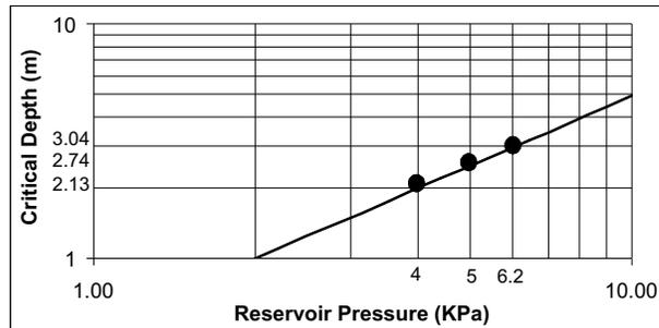
Figure 12 CPC model prediction of critical depth versus laboratory-measured values ( $D=7.8$  mm  $Q_{gs}=0.234$  m/s)
