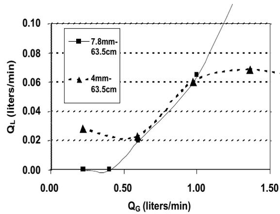
**Figure 6** Liquid versus gas injected ( $D=4$  mm,  $h=63.5$  cm) detail - production characteristic at small laboratory gas injection
