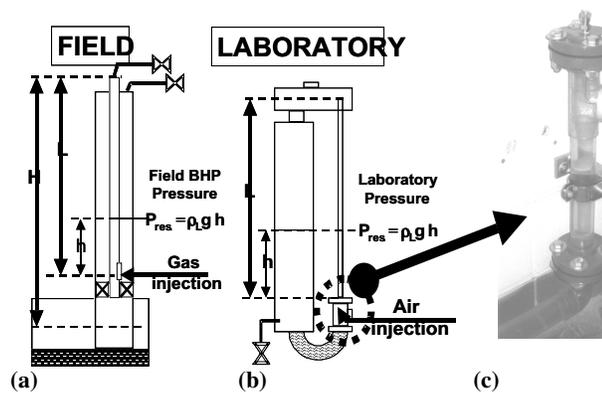
**Figure 3** Schematic of field and laboratory gas lifting (a) Key elements of field gas-lifting . (b) Laboratory (c) gas injector device used in the laboratory (detail).
