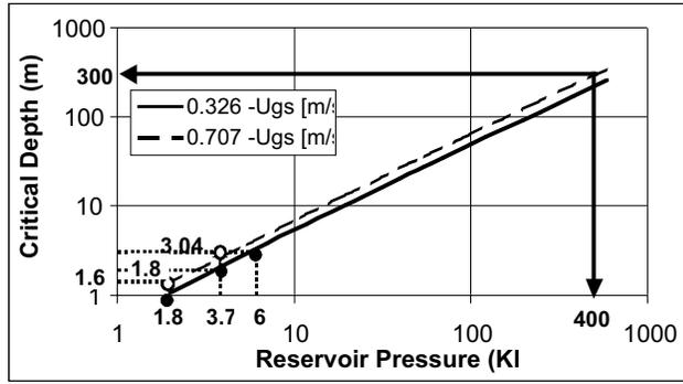
Figure 13 Critical depth versus reservoir pressure (CPC simulated field conditions for  $D=12$  mm,  $U_{gs}=0.33$  and  $0.71$  m/s)
