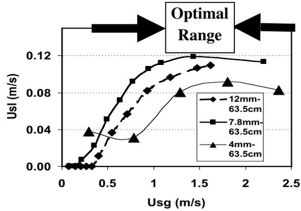
Figure 7 Production characteristics (superficial velocities) for D=4, 7.8 and 12 mm tubes at h=63.5 cm
