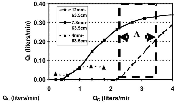
**Figure 5** Liquid production versus gas injected for 12, 7.8 and 4 mm tubes at 63.5 cm fluid level (laboratory).
