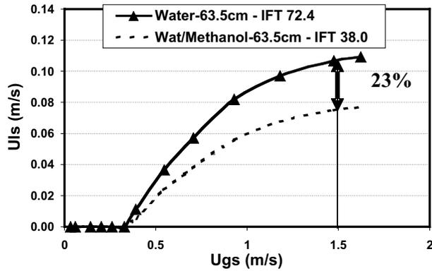
Figure 8 Superficial liquid velocity versus superficial gas velocity for water only and water-methanol (D=12mm, h=63.5 cm)
