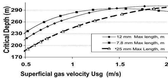
Figure 14 critical depths versus superficial gas velocity for 7.8, 12 and 25 mm tubing (reservoir pressure 400 KPa - 58 psi).
