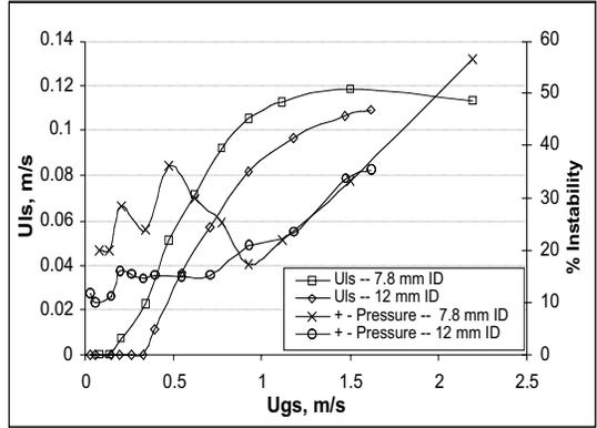
Figure 10 Flow instabilities with water flowing in a 12 mm and 7.8 mm ID tube
