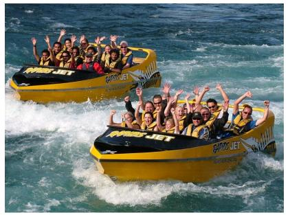
Tour boats feature tiered (staged) seating allowing passengers to see the water conditions ahead. Internal width is maximised for seating. The boats have high sides with good freeboard even at displacement.
