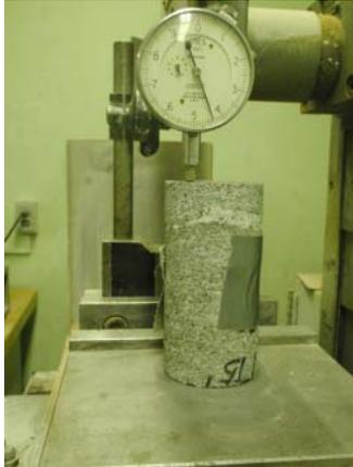
Dial Gage – To measure the tolerance level
