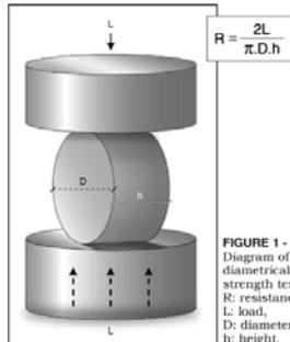
FIGURE 1 - Diagram of diametral tensile strength test. R: resistance, L: load, D: diameter, h: height.
