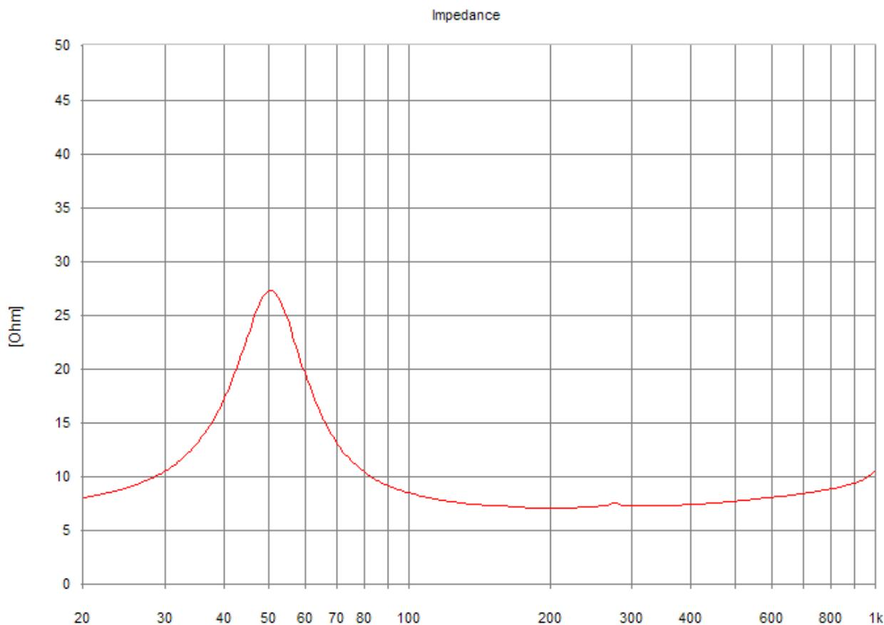
Fig. 1: Impedance plot of 8" driver mounted in enclosure
