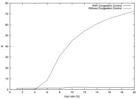
Fig. 3. Average network loss for N cbr sources
