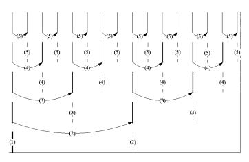
Fig. 4. GOP structure of the video coder
