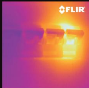
Overheated connection (without MSX)
