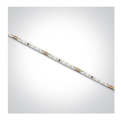
Slim Flexible LED light strip, with SMD2110 LEDs, 196LEDs/meter, 14,4W/meter.Supplied in 5 meters roll with white PCB and double adhesive tape for a better fixing.
