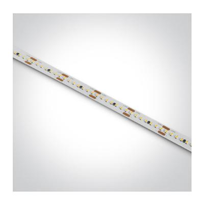
Flexible LED light strip, with SMD2216 LEDs, 238LEDs/meter, 19,2W/meter.Supplied in 5 meters roll with white PCB and double adhesive tape for a better fixing.
