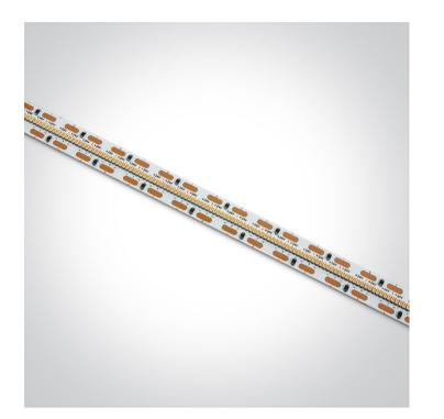
Slim Flexible LED light strip, with SMD2110 LEDs, 700LEDs/meter, 24W/meter.Supplied in 5 meters roll with white PCB and double adhesive tape for a better fixing.
