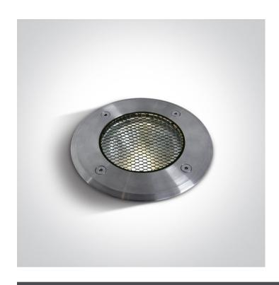
20W COB LED inground with removable honeycomb, IP67, stainless steel 316, for path illumination.
