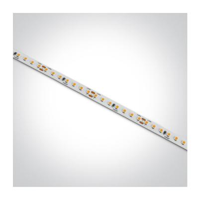
Flexible LED light strip, with SMD2835 LEDs, 140LEDs/meter, 19,2W/meter.Supplied in 5 meters roll with white PCB and double adhesive tape for a better fixing.
