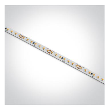
Flexible LED light strip, with SMD2835 LEDs, 140LEDs/meter, 19,2W/meter.Supplied in 5 meters roll with white PCB and double adhesive tape for a better fixing.
