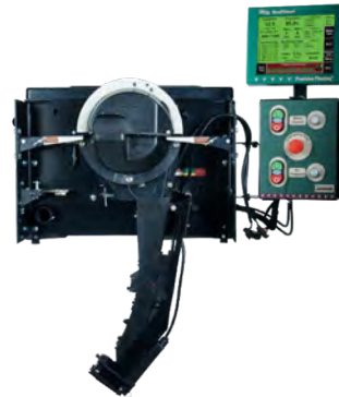
Image: planter singulation unit used in environmental growth chamber trial
