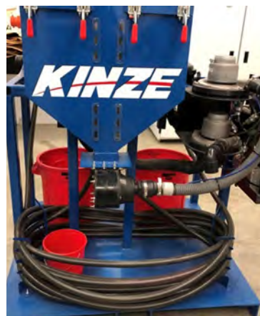
Image: This bulk fill test stand was developed by Kinze Manufacturing to replicate their air seed delivery system. The system includes a small, bulk fill chamber, entrainer, seed delivery tubing (length equivalent to a 24-row planter) and two individual vacuum meters.
