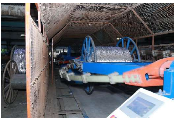
Laying of Cores
