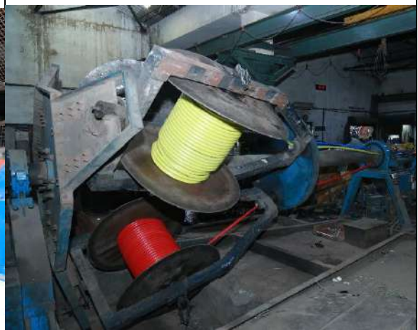
Laying of Cores
