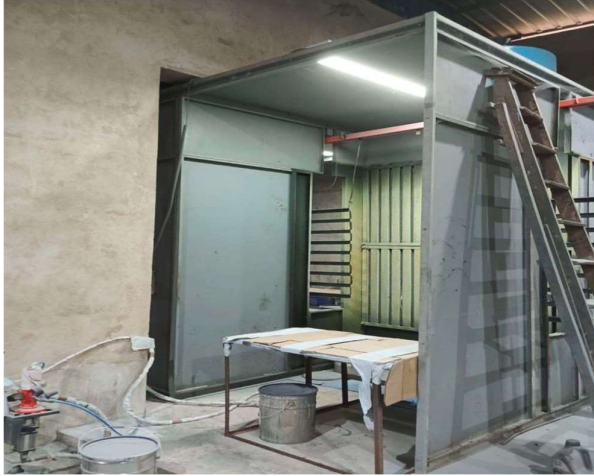
PVDF Coating Machine Unit no 3
