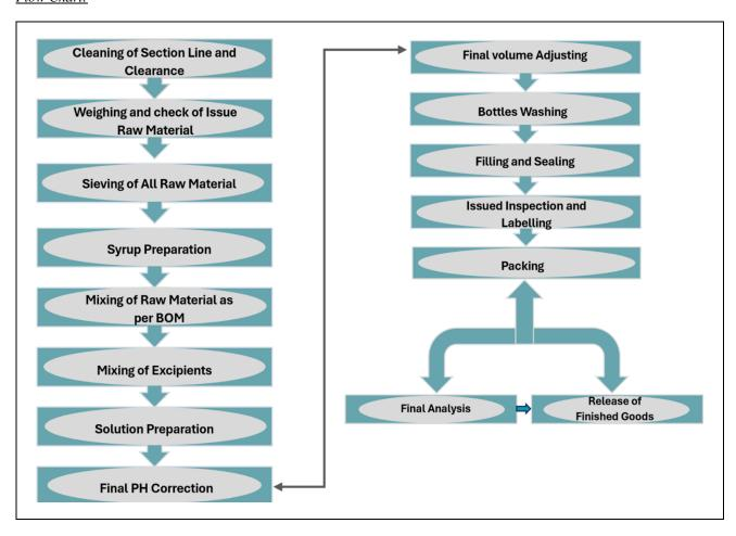
The IPQC section of the Liquid Oral Section conducts online inspections of the solution's pH and the volume of filled bottles. Samples of filled bottles are sent to QC for final analysis, and the filled bottles are placed in finished quarantine. Once QC approves the quality, the product is moved to the BSR (Batch Release Section).
