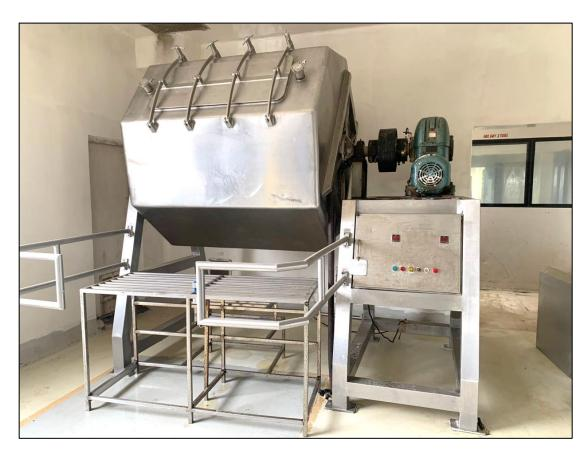
Blender Machine for Dry Granules Mixer
