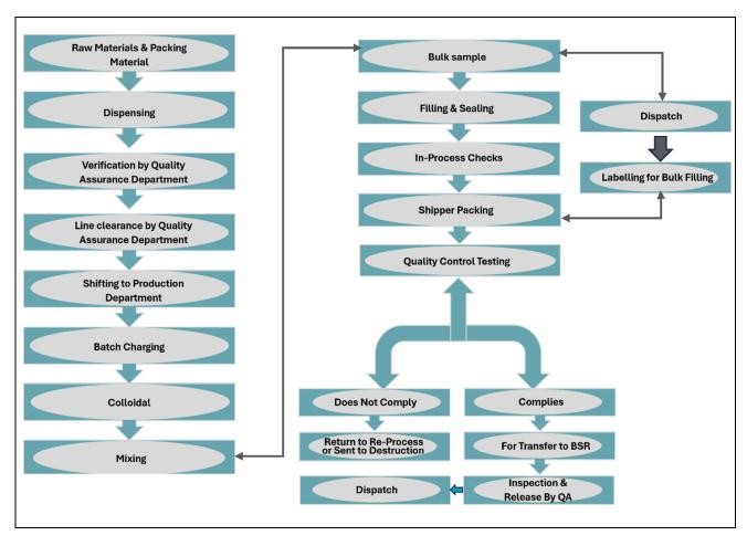
First of all, the Line clearance is must from QA department in order to start the production. The QA department observes all tanks of process and storage physically and washing is performed, and sample of Rinse water is sent from each and every machine in order to check the residue of the old batches. After getting the clearance from the QC that the machines are clean ready to use, the QA department provides the batch Process clearance form the next batch.
