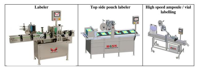
The Labelling machine is used for full/partial Labelling on different size of flat or rectangular containers. The automatic model is equipped with roller spacing device resulting in a simple operation with "No change parts required." These machines are used in pharmaceutical / cosmetics / chemicals / agriculture and many more industries. These machines are used to paste label on the bottles / pouches / vials etc.
