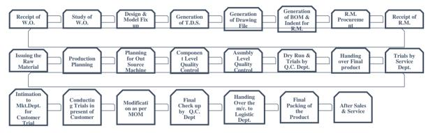
Our process for manufacturing machines starts after our marketing and sales team finalizes the machine dispatch schedule with the customer. Thereafter, the material requirement planning is calculated, following which the parts delivery schedule is sent to relevant suppliers and in-house manufacturing unit.
