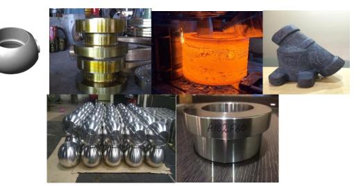
Manufacturing of valve components is be done from a wide variety of materials depending on the application by the client. All Forgings such as Body, Adaptors, Balls, Stems, Trunnion Plates, Seat Rings Bonnets, and Y-Strainer Forgings are manufactured and supplied in proof machined condition.
