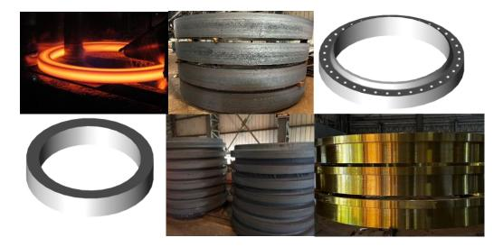
The process starts with a circular preform of metal that has been previously upset and pierced (using the open die forging process) to form a hollow "doughnut" This doughnut is heated above the recrystallization temperature and placed over the mandrel roll. This mandrel roll then moves under pressure toward a drive roll that continuously rotates to reduce the wall thickness, thereby increasing the diameters (I.D. and O.D.) of the resulting ring.
