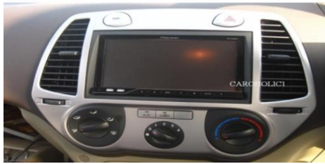
TFT Display with no touch option
