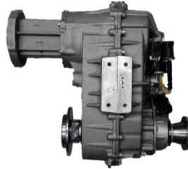
Dual – offset Transfer Case with bevel differential
