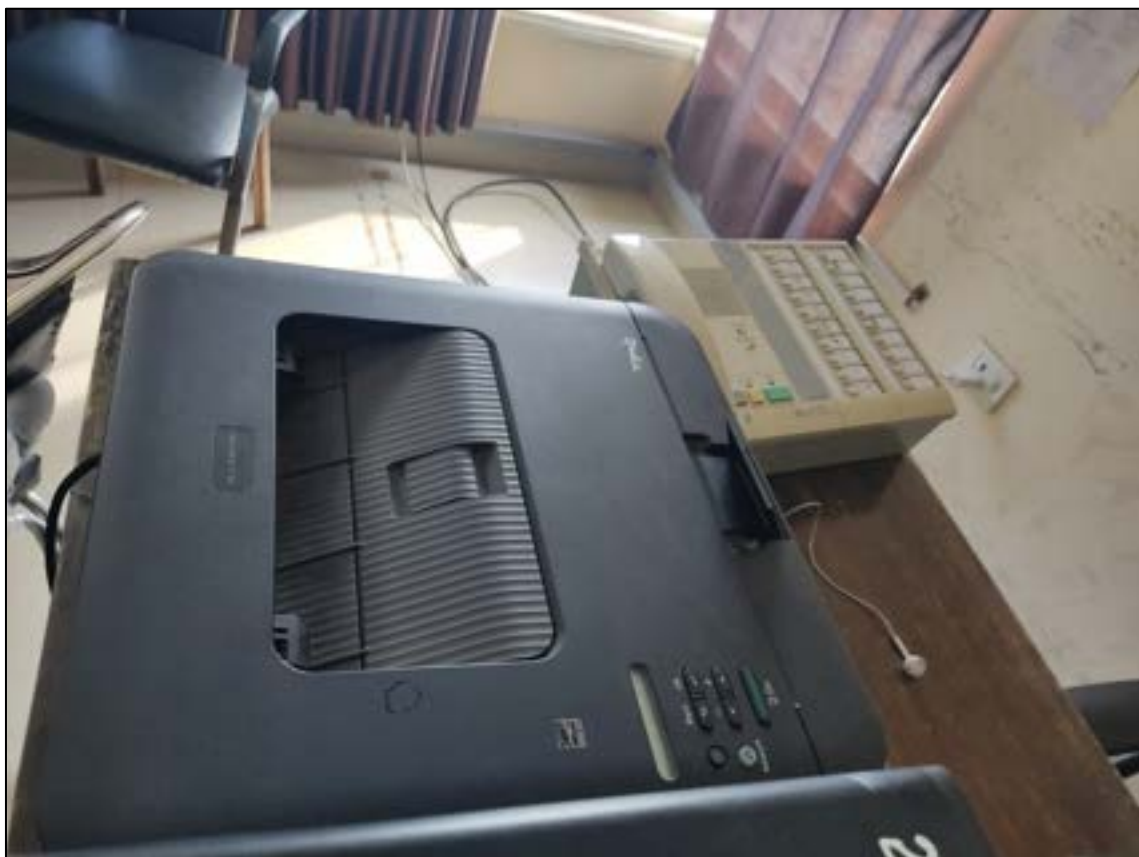
Figure 9-16 Network Printer and Intercom Master Unit at control room
