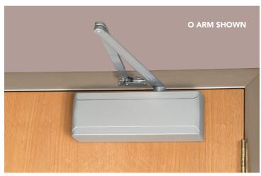
The standard application of the 281 door closer is the most common providing high degree of door control and range of power adjustment. The closer is mounted on the pull side of the door with the arm mounted on the face of the frame. When the door opens, the arm passes over the top of the door.
