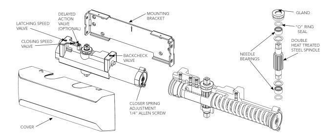
The 281 Series complies with ADA for reduced open forces of 5 lbs. for interior and 8 lbs. for exterior doors.
