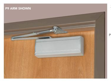
Parallel Arm Application – The 281 closer is mounted on the push side of the door. As the door opens, the closer swings with the door and gives full headroom in the door opening. Other advantages are that the closer arm does not project into the room, the frame can be quite narrow and the door can be swung open much further than in Top Jamb Applications. However, the closing force is not as great.
