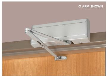
Top Jamb Application – The 281 closer is mounted on the frame face above the door. The foot is mounted on the push side of door. This application is for use on exterior doors opening out to protect the closer from the weather. The Frame Face must be at least 4-3/8". With the 281-B mounting plate, the rail must be at least 1-7/16" min.
