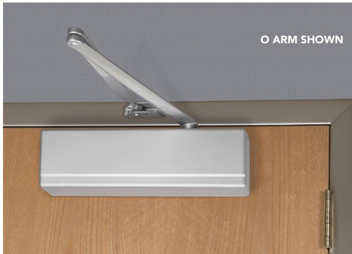
The standard application of the 351 door closer is the most common and the most desirable. The closer mounts on the hinge (pull) side of door (except when the W Corner Bracket is used). **Note:** This application is not recommended on exterior doors (the closer is not protected from weather). The cover projection normally limits the door opening to a maximum of 160°.
