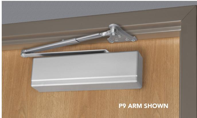
**Parallel Arm Applications** - The 351 closer is mounted on the push side of the door. As the door opens, the closer swings with the door and gives full headroom in the door opening. Other advantages: the closer arm does not project into the room; the frame can be quite narrow and the door can be swung open much farther than in Top Jamb Applications.
