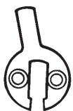
Std Cam (13-0664) for all functions except for 50 and the Inside cam for 16 function locks
