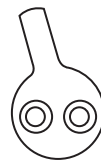
Std 6300 Cam for all functions except for 50 and the Inside cam for 16 function locks
