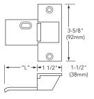
Full mortised Dimension "L" equals door thickness plus 1/2" (13mm).
