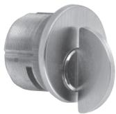
Classroom function cylinders have a pin to block cam rotation in the locking direction. The pin may be installed on either side of the cam, depending on the hand of the door.
