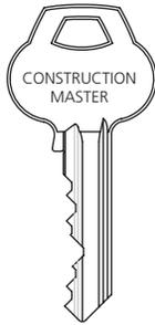
The construction master key operates all Corbin Russwin cylinders while the building is under construction. Upon completion of the construction phase, it can be voided without removing the cylinders from the locks, simply by turning the change key in each cylinder. Construction master keying is not available for interchangeable core. Temporary cores are available for IC jobs that require construction keying.
