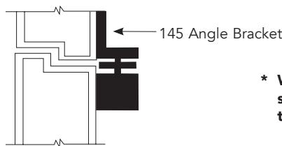
\* When using vertical rod exit devices and or surface/flush bolts, use caution in choosing the proper size to ensure compatibility
