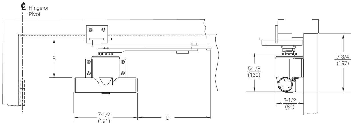
Body mounting holes are spaced 4-1/8" (105mm) horizontally and 1-3/8" (76mm) vertically.
