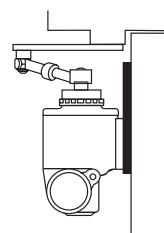
**Narrow Top Rail - 1988 Drop Plate:** For use where a narrow top rail prevents the closer from being mounted directly to the door surface.
