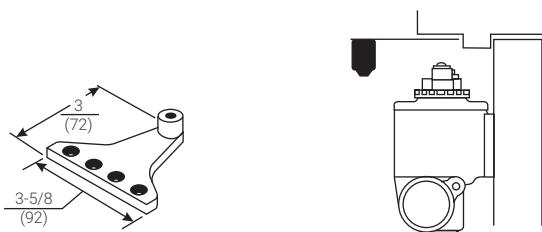
**Mounting Between Doors - 413A Soffit Bracket:** For use where insufficient space between companion doors does not permit use of other soffit plates. This bracket permits mounting of the closer between doors with as little as 4-1/8" (105mm) of header space. Permits closer arm to clear up to a 5/8" (16mm) high stop.
