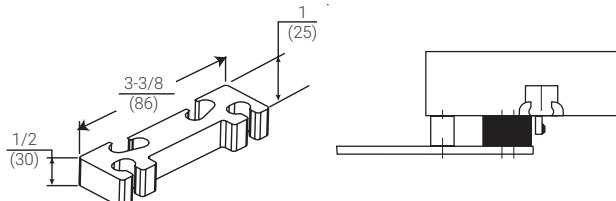
**Clearance/Support Blade Stop - 891 Spacer Block:** For use where the frame has a blade stop and the soffit plate must be mounted on the frame rabbet. This accessory is used in combination with the standard Spacer Block to provide clearance of the blade stop.
