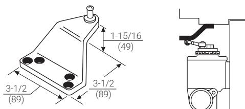
**Flush Transom - 589L Angle Bracket:** For use where rabbeted or flush transom conditions prevent installation of a soffit plate. Used in combination with the 289 soffit plate, or it may be used in combination with the 290 soffit plate when it is necessary for the closer arm to clear a separate overhead door holder.
