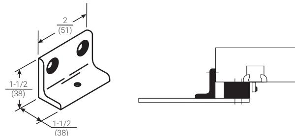
**Narrow Frame - 890 Support Bracket:** For use where the frame is narrow, and the soffit plate cannot be mounted directly to the frame soffit or rabbet. Used in combination with the 891 Spacer Block on blade stop frames to provide extra support and needed clearance of the blade stop.
