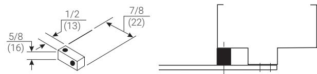
**Flush Transom - 293L Angle Bracket:** For use where flush transom conditions prevent installation of the standard hold open soffit plate. Used for parallel hold open arms.
