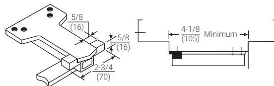
**Wide Frame - 6191 Reinforcing Kit:** Optional for use with all parallel arm UNI Stop door controls. Used to support the soffit plate on installations with wide frames. Clamps may be used with or without the spacer block, depending on frame conditions.
