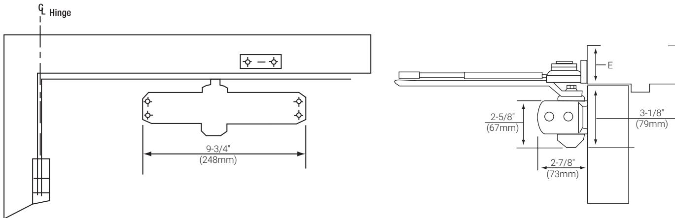
Mounting holes for closer body are spaced 3/4" (19mm) vertically x 9-1/16" (230mm) horizontally.
