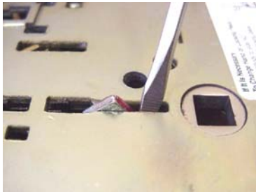
Step 3. Push on edge of Locking Piece between Locking Piece and Square Spindle Hole. Rotate 180°. Red mark indicates locked side of door and MUST be seen on either side of lock.
