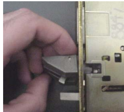
Step 4. Rotate Latchbolt 180 0 to desired handing position.
