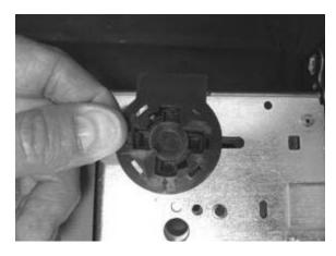
9. Gently press Cylinder Monitoring Assembly into cylinder hole on the new side of the lockbody.
