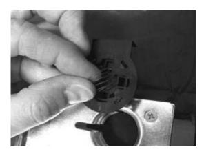
Remove Inner Shell from Outer Shell by gently pressing the Inner Shell upwards from the bottom.
