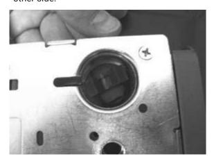
Turn the Inner Shell on its side and slide it down into the Outer Shell.
